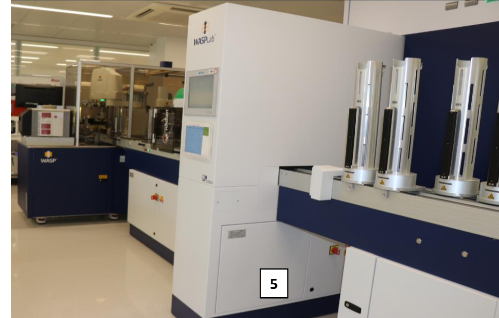
5) WASPLab® AST Line : AST plates are digitized after 16 hours of incubation
